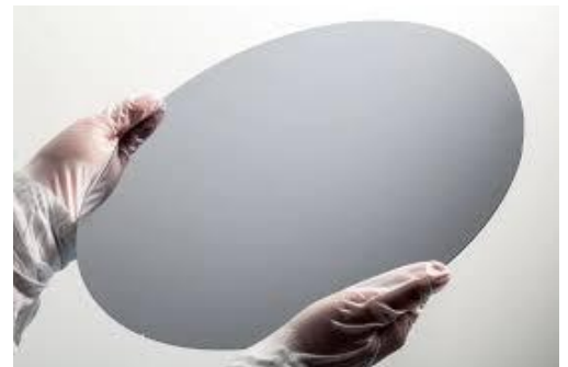
300mm Wafer, Polished Surface
